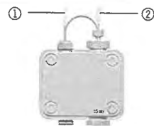
Fig.19 Flushing rear piston area
