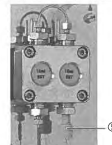
Fig. 8 Solvent line on pump head
