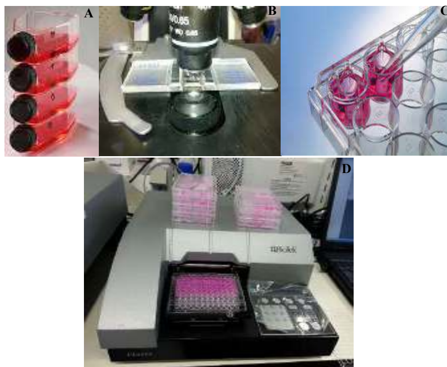
Figure 25. Cytotoxicity: A- Cell suspension; B- Cell counting; C- Cells with sample; D- Absorbance at 540 nm.
